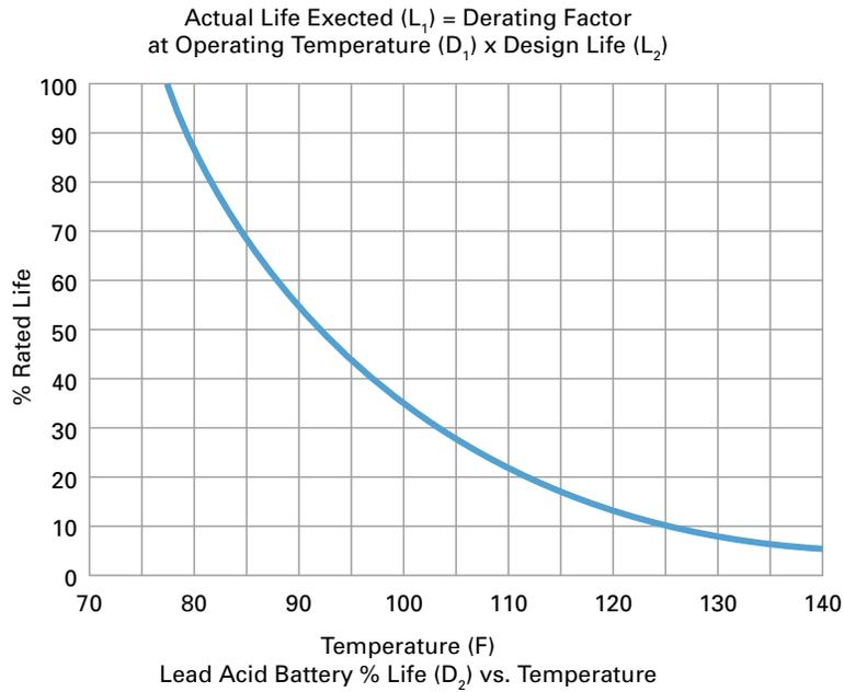
Based on the equation Actual life = Derate factor x Design Life, a VRLA battery with a design life of 10 years, operating at 85 degrees F, per the graph, will have an actual life of 6.9 years (6.9 = 69% of 10).
